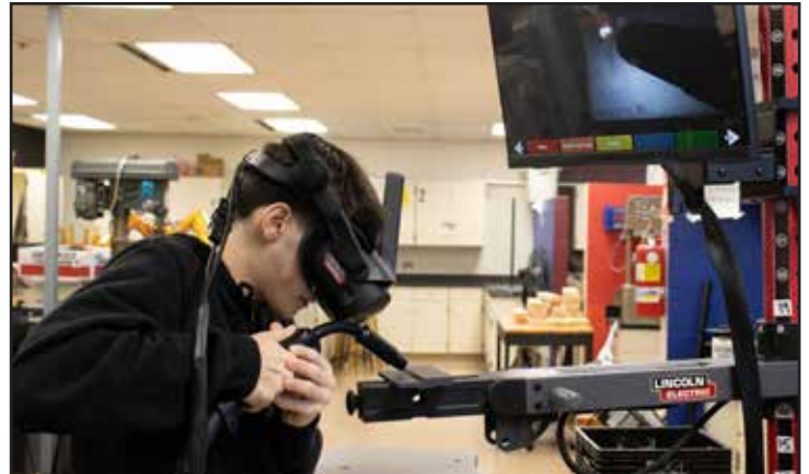
IMPE student, Chase Wheaton (Stow-Munroe Falls), gains welding experience on the virtual reality simulator
